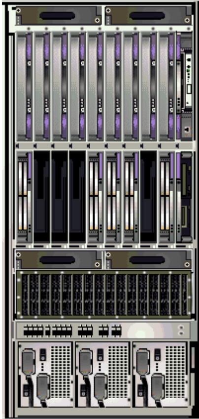
FIGURE 5-2 Sun Fire 15K/12K Platform Physical View—Front
