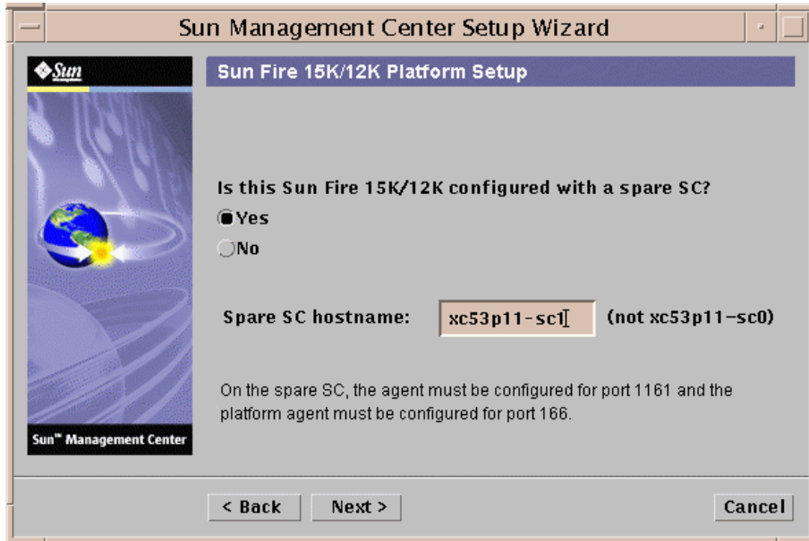
FIGURE 2-5 Spare System Controller Query
