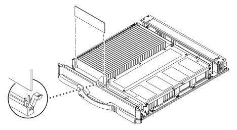
6. Holding the DIMM by its edges, remove it from the slot and place it on the ESD mat.
