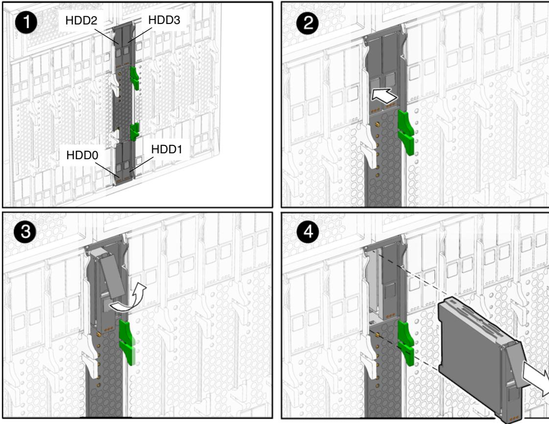
**FIGURE 3-2** Hard Drive Locations, Release Button, and Latch
