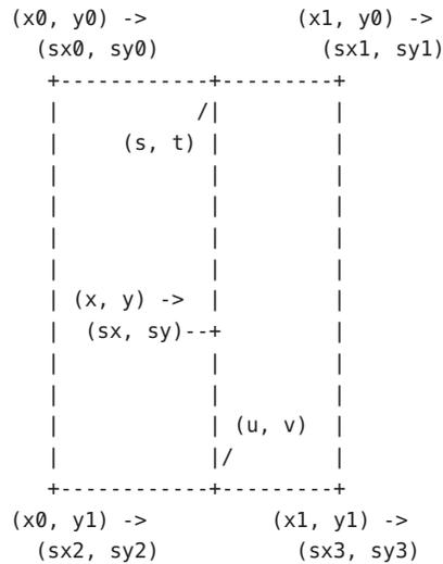
The results of above interpolation are shifted by  $(-postShiftX, -postShiftY)$  to produce the source pixel coordinates.
