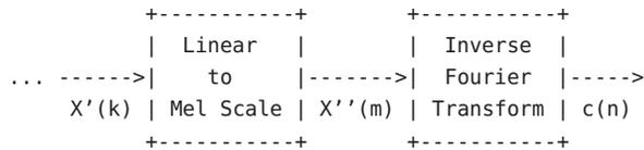
where  $X'(k)$  is defined in linear frequency scale and  $X''(m)$  is defined in mel frequency scale.
