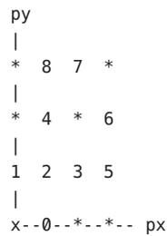
where x marks the start point of a path segment, the numbers are the values of the chain code for the segment that ends at the point.
