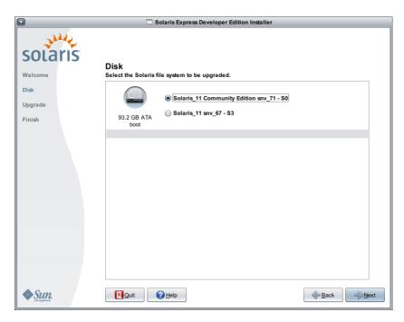
This panel displays the internal disks, external disks, and solid-state drives that are available on the system. To be recognized by the installer, the disks and solid-state drives must be turned on at the time the computer boots.
