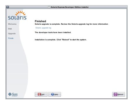
The final panel displays completion messages. You can review upgrade logs in this panel. You can either Quit or Reboot from this panel.
