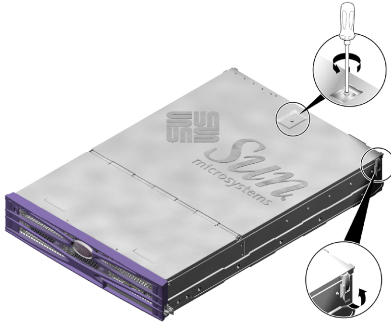
FIGURE 1-4 Location of Captive Screw and Side Catches on Back Section of the Cover
