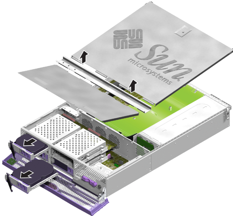
FIGURE 1-21 Removing Cover Assembly and Hard Drives to Access Interface Boards
