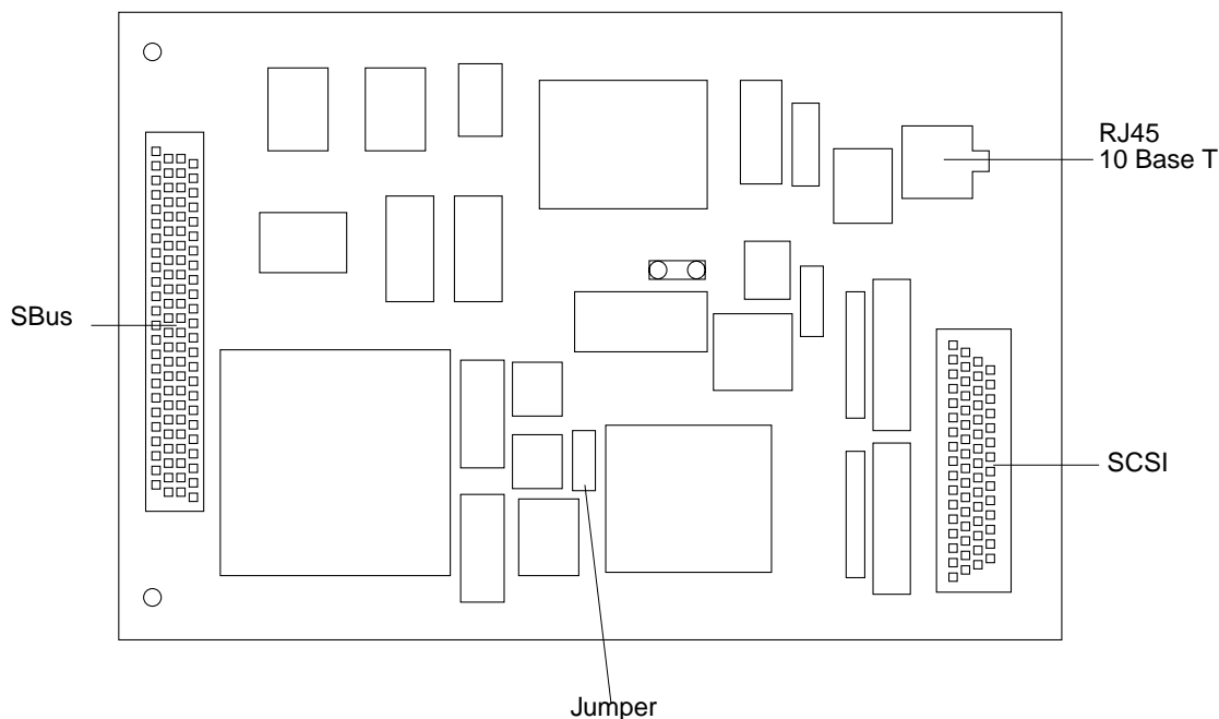
Figure A-3 FSBE/S SBus Card Jumper
