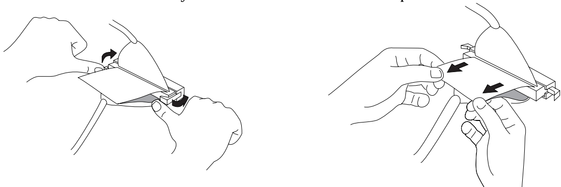
Figure 9-13 Releasing Ejectors and Disconnecting the SCSI II Cable
