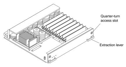
3. Pull the ends of both extraction levers outward, then gently pull the board out of the card cage.
