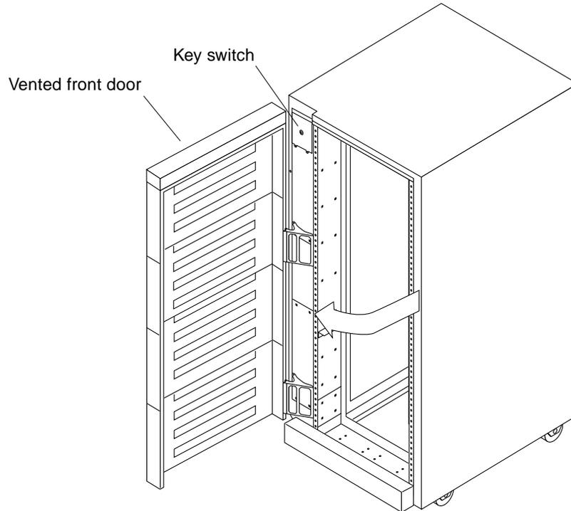
Figure 2-1 Opening the Front Door of the Cabinet
