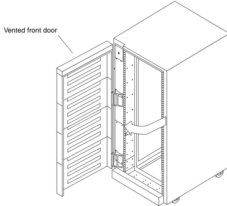
*Figure 4-1* Opening the Vented Front Door
