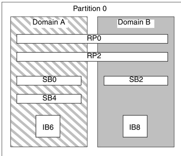
**FIGURE 1-3** Sun Fire E4900/4810/4800 Systems in Single-Partition Mode
