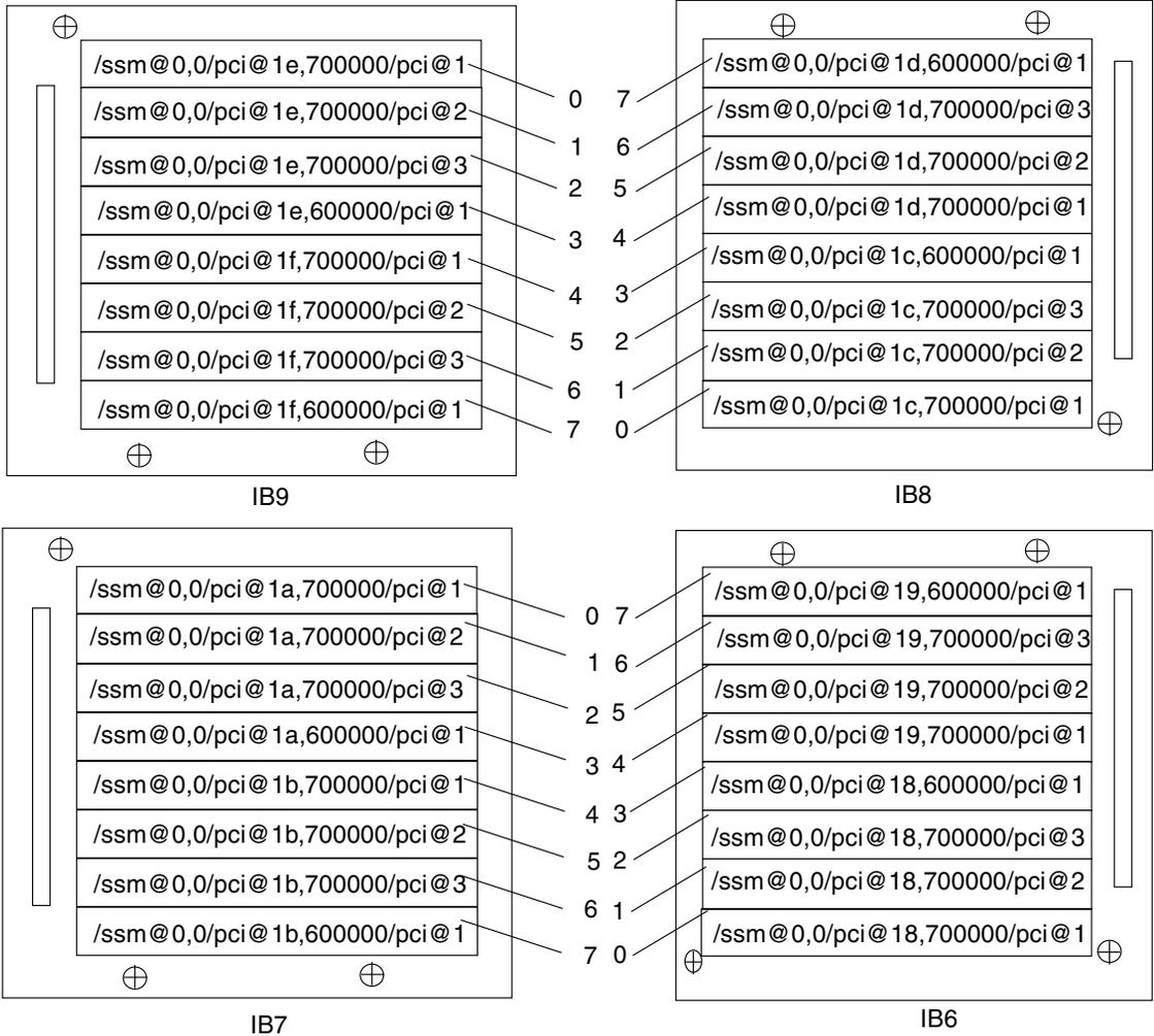
Note: Slots 0 and 1 of IB6 through IB9 are short slots.
