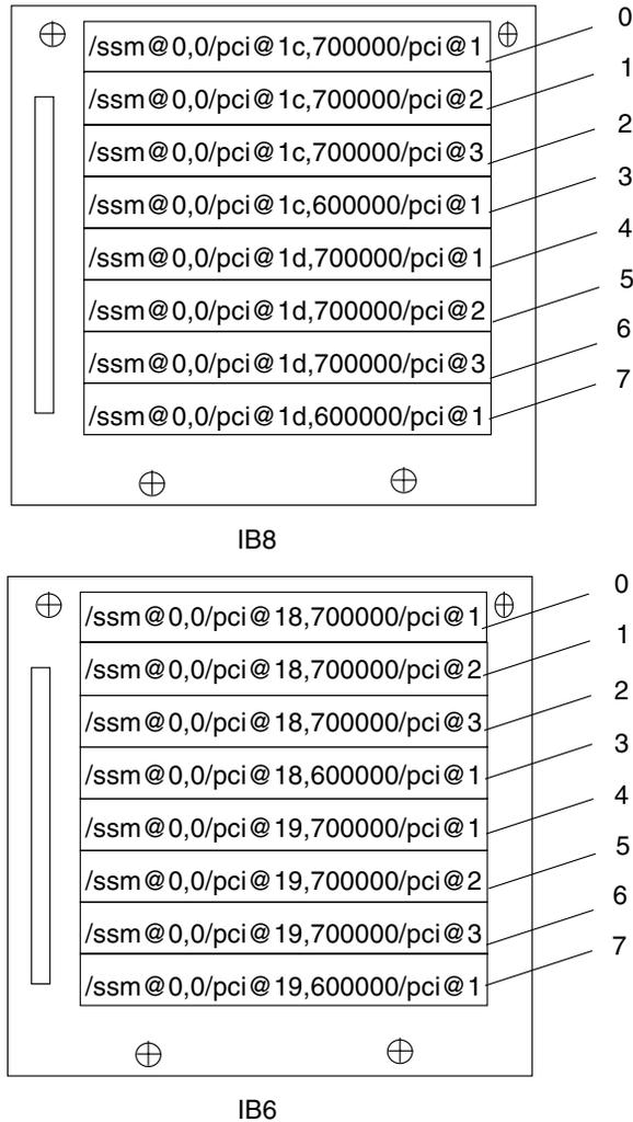
Note: Slots 0 and 1 for IB6 and IB 8 are short slots.
