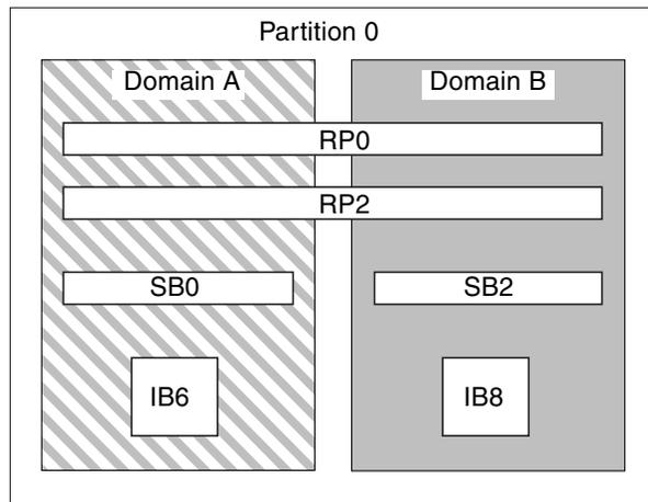
FIGURE 1-5 Sun Fire 3800 System in Single-Partition Mode
