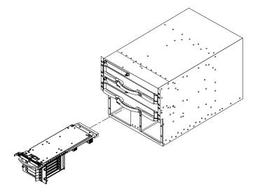
8. Dynamically reconfigure the I/O assembly back into the system.
