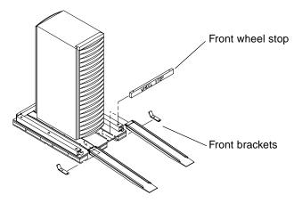
**Note** – The brackets can be used later to bolt the cabinet to the floor.
