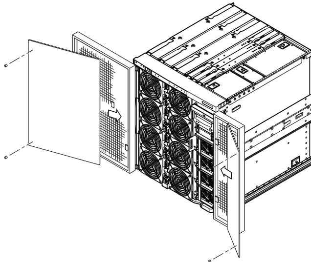
2. Install the new filters and replace the plastic pins.
