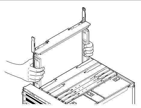
c. Slowly push down from the center top of the CPU/Memory filler board as shown below, until the top face of the board is approximately three to four inches from the top of chassis.
