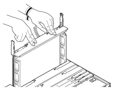
d. When the board is approximately three to four inches inch from the top of the chassis, change your grip and grasp the ejector levers so that they are oriented in the vertical position, 90 degrees straight out from the board.
