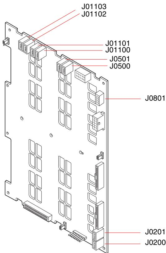
The locations of the connectors on the PCI Dual Fibre Channel Network Adapter+ are shown in the following figure.
