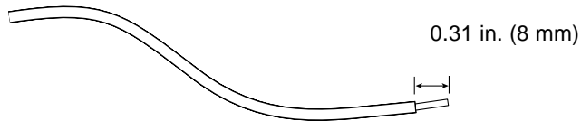
FIGURE 3-2 Stripping the Insulation From the Wire
