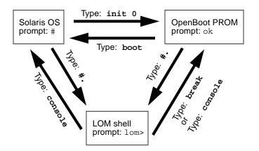
FIGURE 2-1 Navigation Between Consoles
