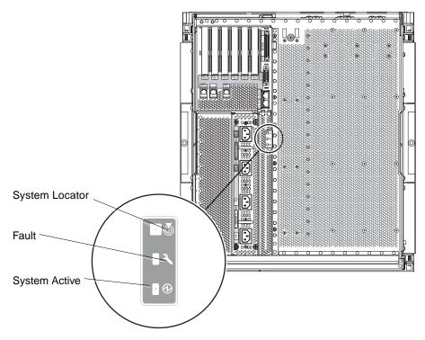
FIGURE 4-2 Server Rear Panel LEDs
