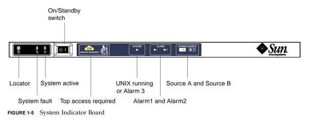
The indicator LEDs function as shown in TABLE 1-2.
