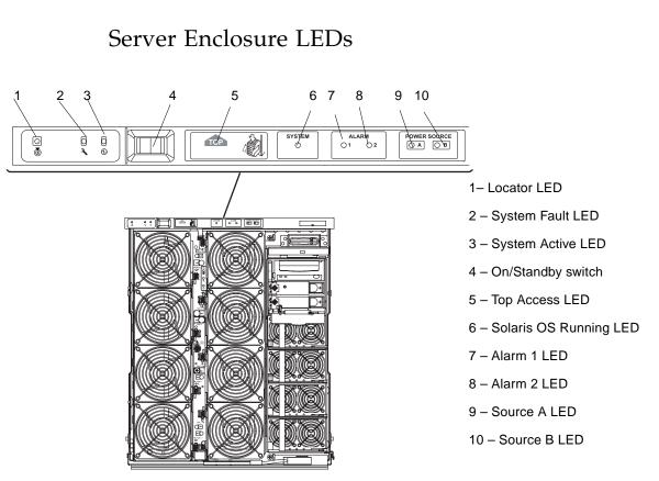
FIGURE 4-1 Server Front Panel LEDs
