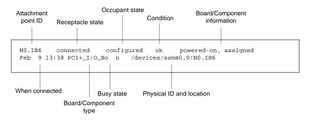
FIGURE 2-2 Details of the Output for the cfgadm -av Command
