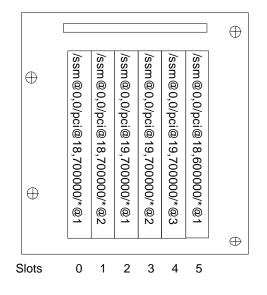
FIGURE D-1 Netra 1290 Server IB\_SSC PCI+ Physical Slot Designations for IB6
