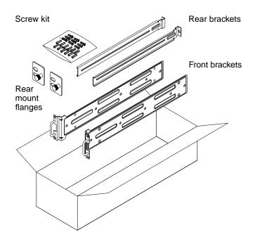
Refer to the Netra 240 Server Installation Guide for the contents of the screw kit.
