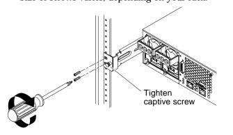
**Note** – For complete instructions on mounting the server in a rack, refer to the *Netra 240 Server Installation Guide*.
