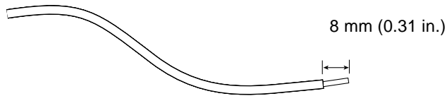
FIGURE 3-2 Stripping the Insulation From the Wire
