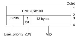
FIGURE 5-2 Ethernet Tag Header Format
