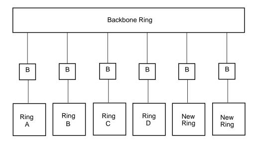
In the configuration illustrated above, new rings can be added to the Backbone Ring by adding one bridge for each new ring that is added.
