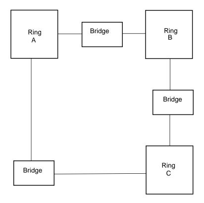
A disadvantage to this loop configuration is that each ring should be bridged to every ring on the network to for maximum performance and connectivity.
