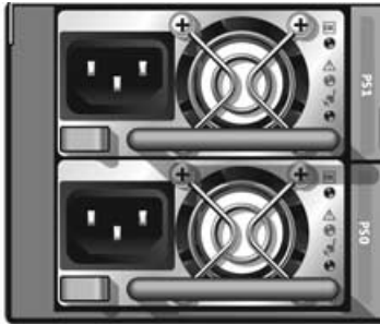
FIGURE 6-4 Rear Panel Power Supplies
