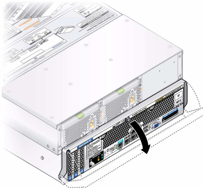
4. Pull the system controller out of the chassis. See [FIGURE 3-31](#).
