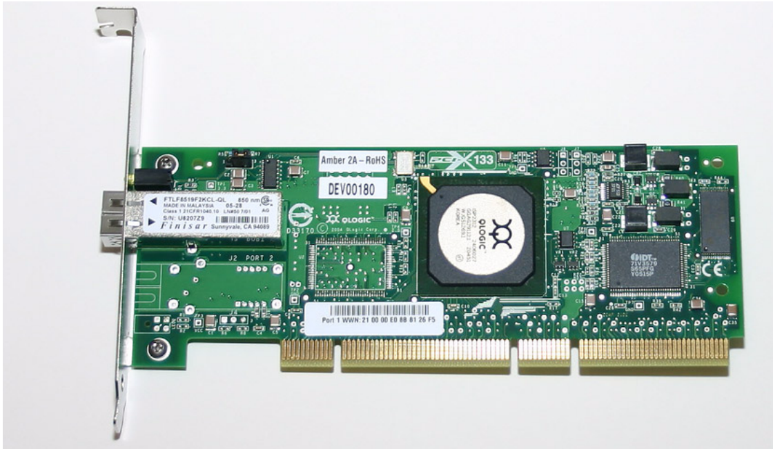
FIGURE 3 Sun StorageTek PCI-X Enterprise 2 Gb FC Single Port HBA (Dust Covers Removed)
