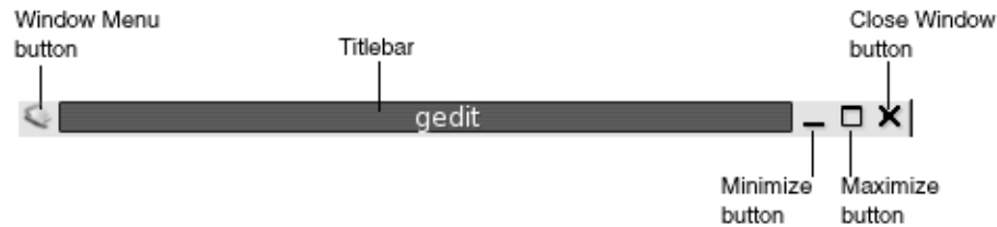
FIGURE 2-2 Top Edge of Frame for a Typical Application Window
