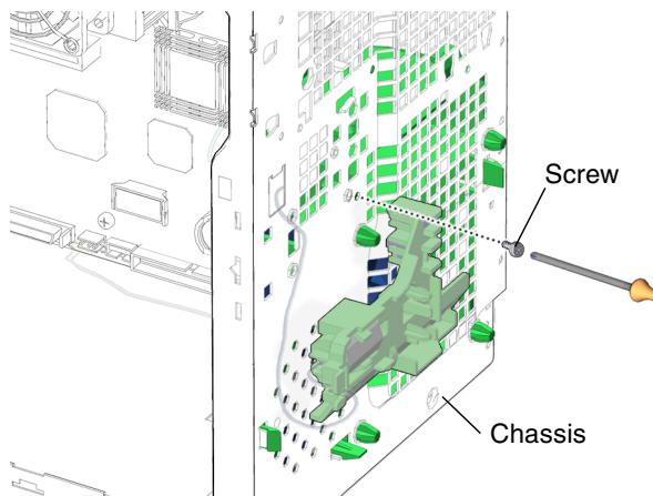
FIGURE 13-41 Installing the Screw for the Front Fan Bracket
