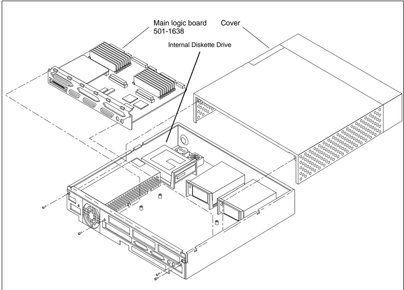
Figure 3-1 Exploded View of the System Unit
