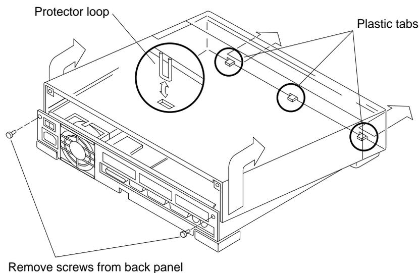
Figure 1-2 Removing the Cover Panel
