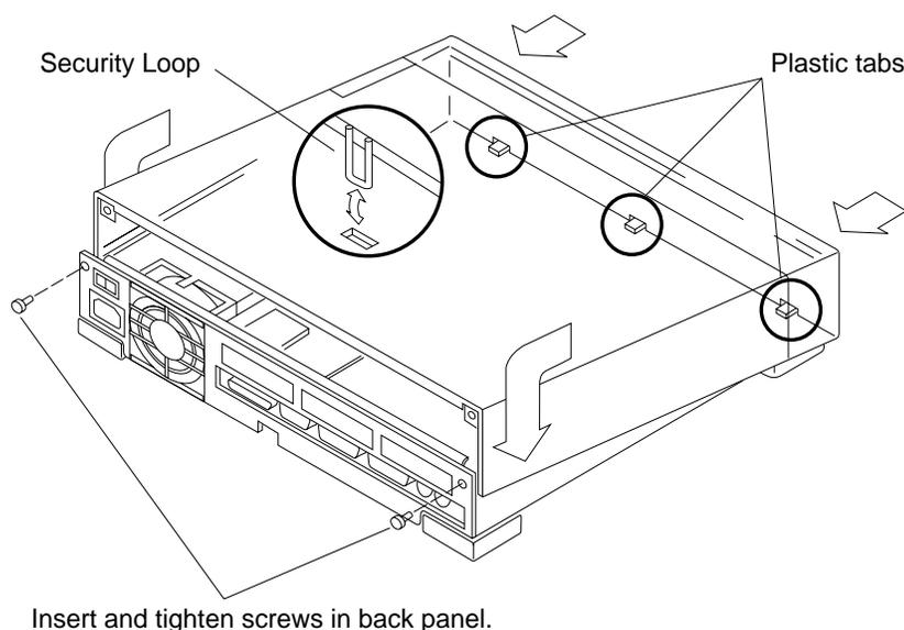
Figure 2-9 Replacing the Cover on the System Unit
