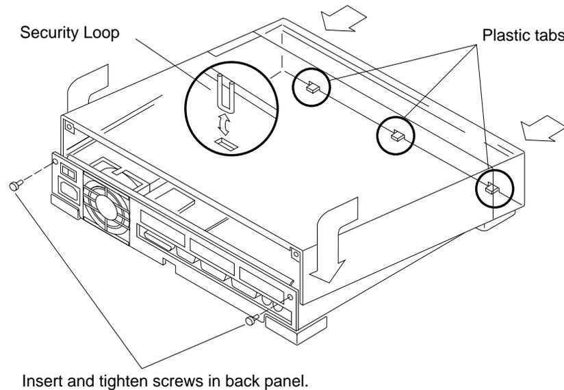
Figure 3-5 Replacing the Cover on the System Unit
