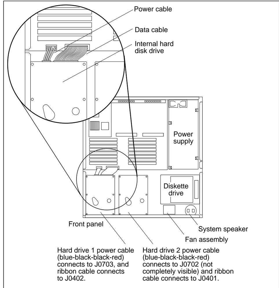
Figure 2-8 Connecting Power and Data Cables to the Hard Disk Drive
