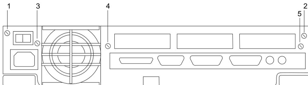
Note: There are five screws on the back panel. Remove screws 1 and 2. Do not remove screws 3, 4, and 5.
