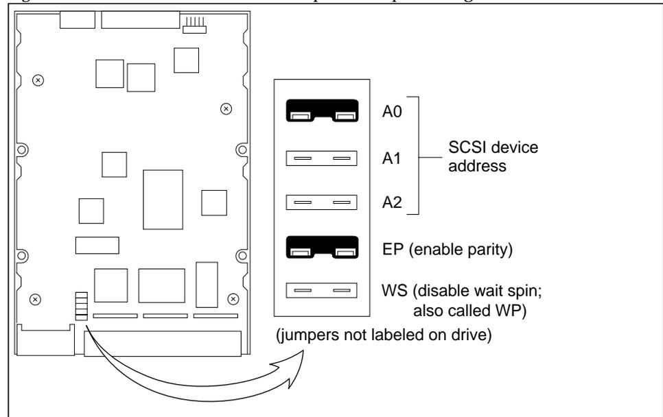
**Figure 2-6** Hard Disk Drive with 5 Jumpers—Jumper Setting for Drive 2
