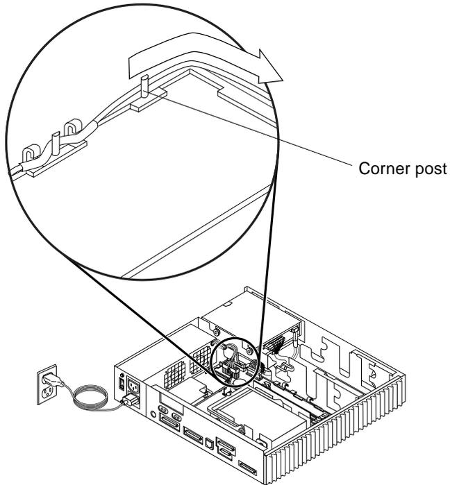
**FIGURE 9-19** Routing the Audio Cable Around the Corner Post
