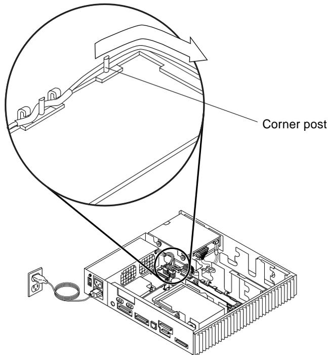
**FIGURE 11-18** Routing the Audio Cable Around the Corner Post
