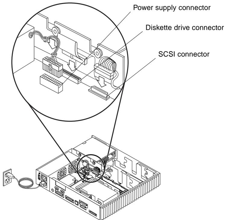
**FIGURE 9-22** Reconnecting the Main Logic Board Connectors
