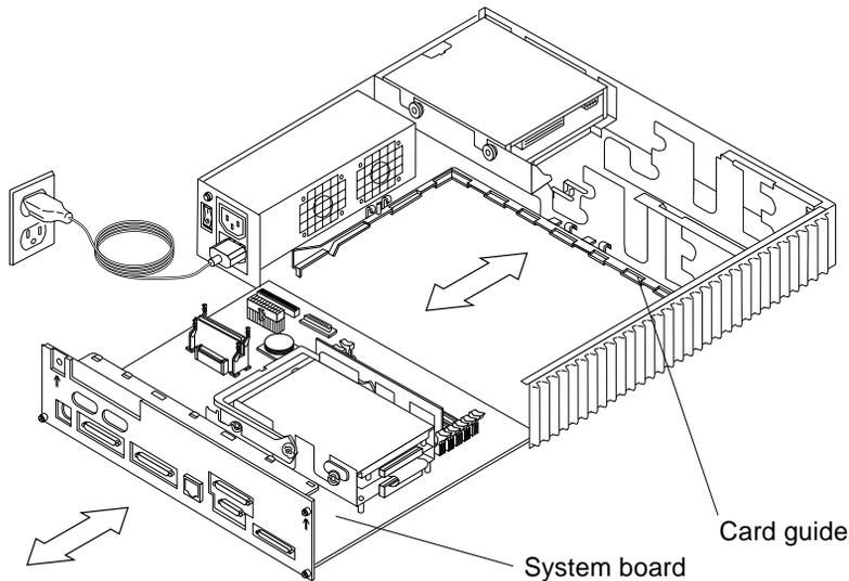
FIGURE 11-29 Removing the System Board
