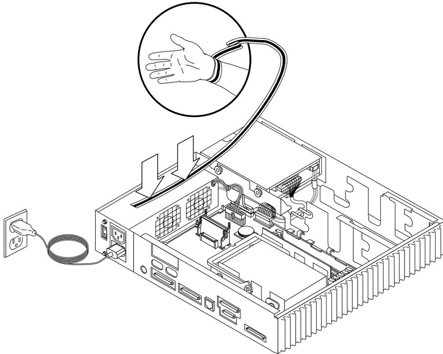
FIGURE 7-3 Grounding the Wrist Strap to the Power Supply
