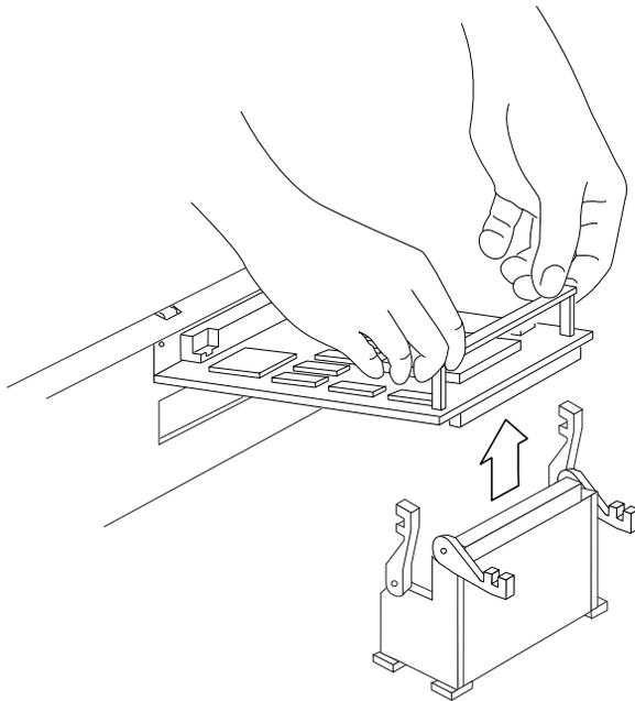
**FIGURE 11-5** Removing the SBus Card
