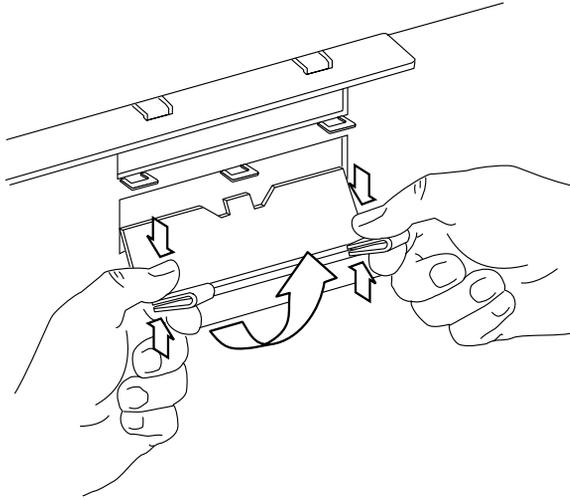
**FIGURE 11-13** Removing the Audio Module Filler Panel
