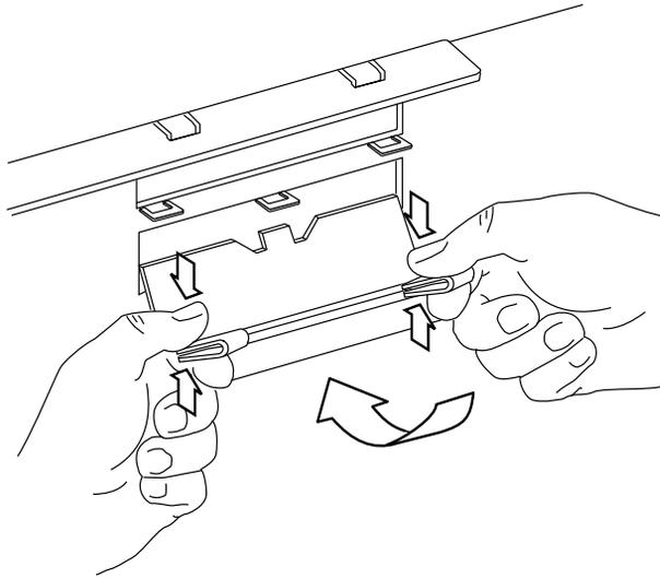
**FIGURE 11-12** Inserting the Audio Module Filler Panel
