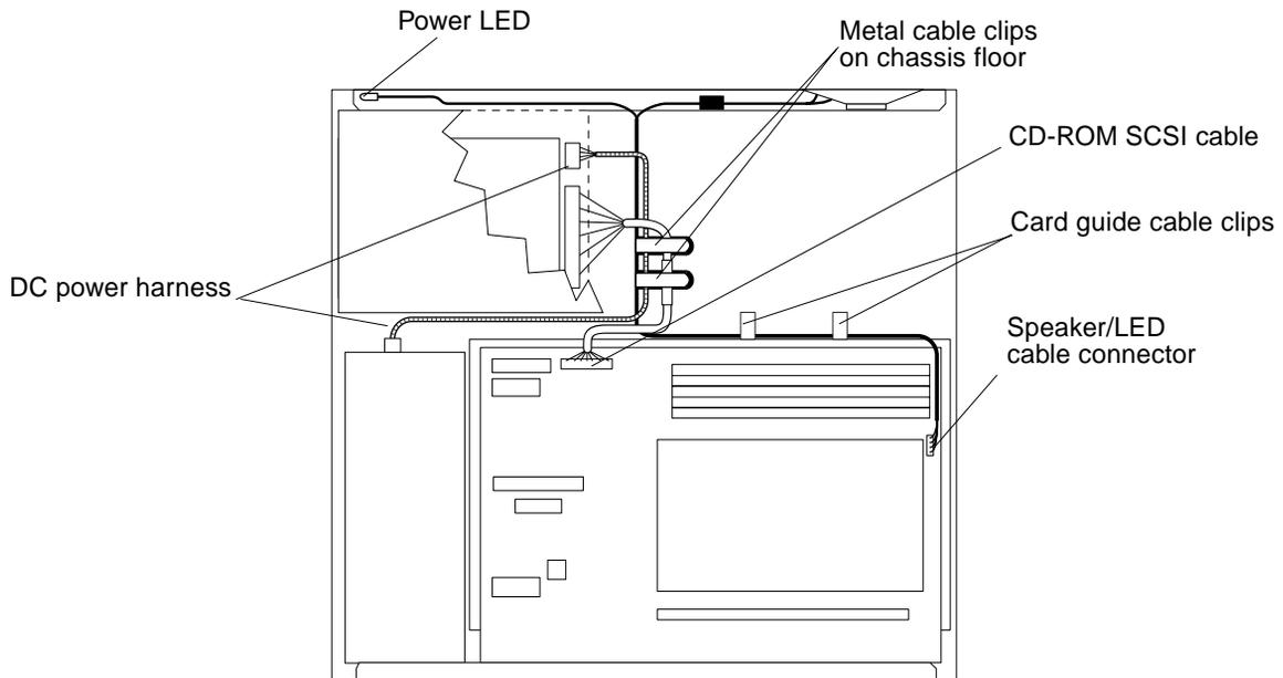
**FIGURE 8-3** Power LED and Speaker/LED Board Cable Connectors
