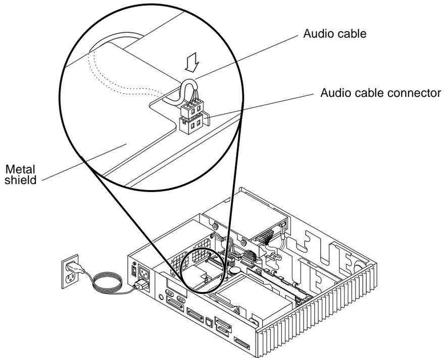
**FIGURE 11-16** Connecting the CD-ROM Audio Cable
