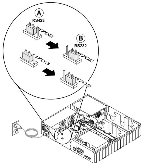
FIGURE 11-32 Setting the Serial Port Jumpers
