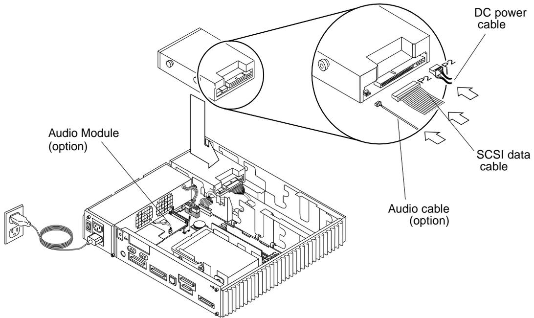
**FIGURE 9-6** Replacing the CD-ROM Drive
