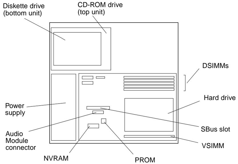
FIGURE 1-2 Interior View of SPARCstation 4 System
