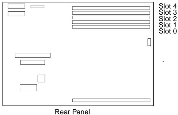
FIGURE 11-19 DSIMM Slot Locations on the System Board
