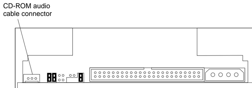
**FIGURE 9-15** Audio Cable Connector on the CD-ROM Drive
