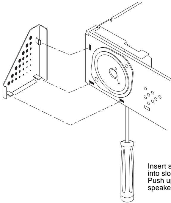
Insert small, flat-blade screwdriver into slots on underside of chassis. Push up on tabs to disengage speaker cover.
