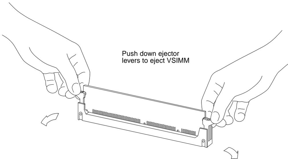
**FIGURE 11-24** Ejecting the VSIMM
