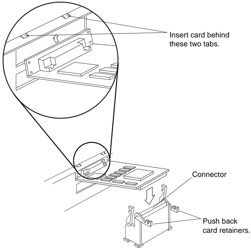
**FIGURE 11-6** Inserting the SBus Card
