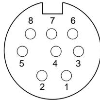
**FIGURE B-6** Keyboard/Mouse Connector**TABLE B-6** Pinout for Keyboard/Mouse Connector
