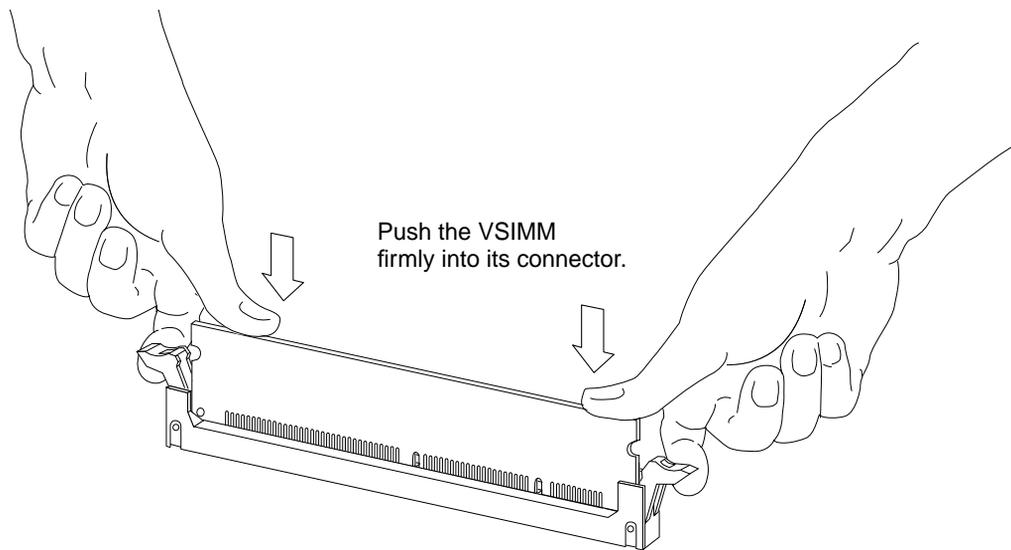
**FIGURE 11-26** Installing the VSIMM
