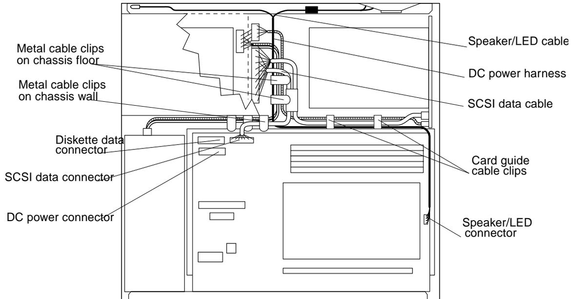
FIGURE 9-13 Internal Cable Routing
