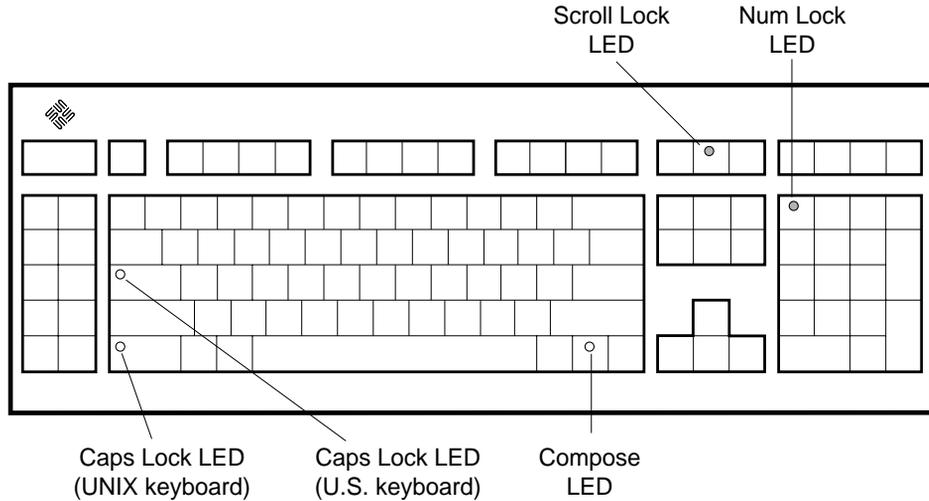
**FIGURE 3-1** Arrangement of Sun Type-5 Keyboard Diagnostic LEDs
