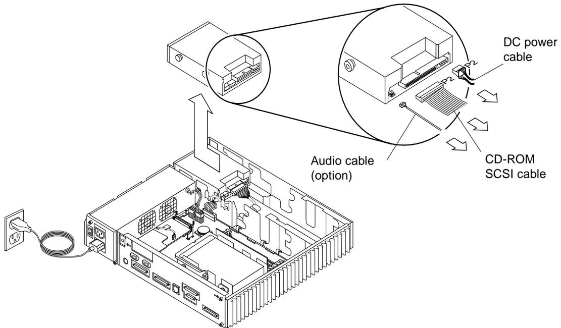
FIGURE 9-4 Removing the CD-ROM Drive
