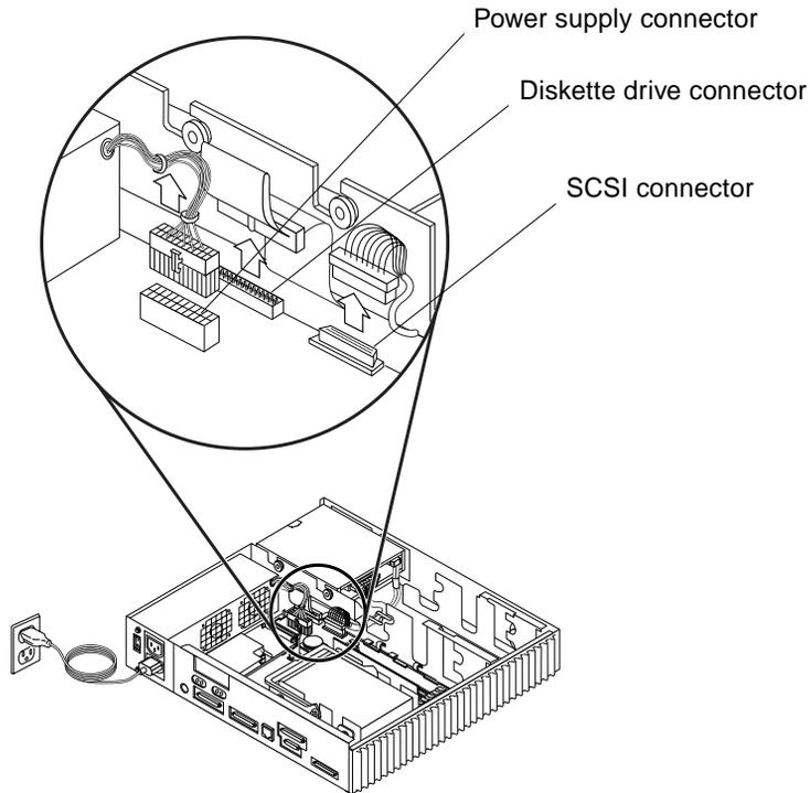
FIGURE 9-17 Disconnecting the System Board Connectors
