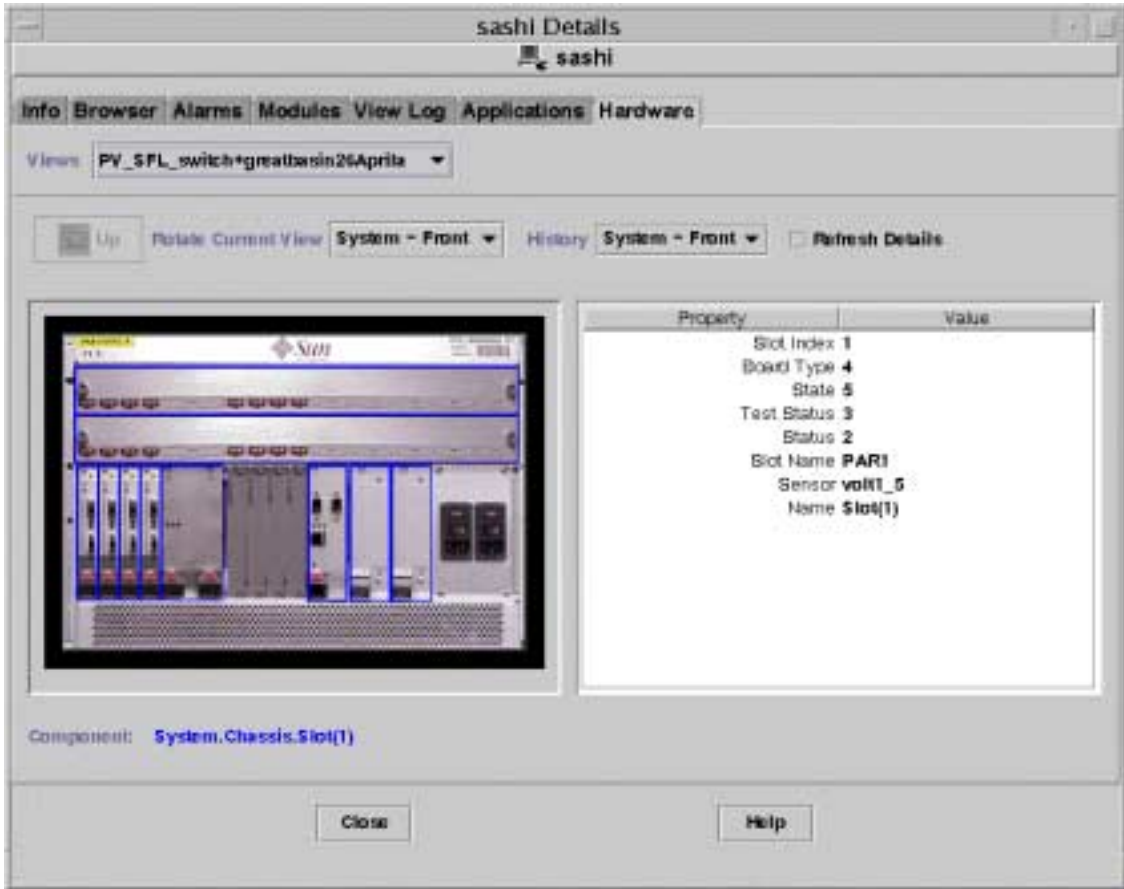
FIGURE 9-15 Physical View of Switch Slot 1
