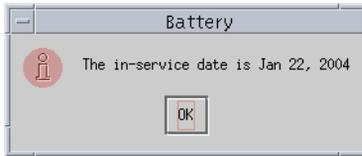
Sun StorEdge Configuration Service sets the in-service date and displays the date in the In-Service Date field in the Battery Information window.
