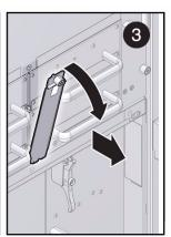
**Note** – Discard the bent hinge pin. Use a new hinge pin in Step 6 below.
