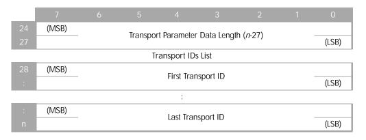
Transport Parameter Specifies the number of bytes of Transport IDs to follow. The Parameter List Length in the CDB contains all the bytes specified in Transport Parameter Data Length. Data Length
