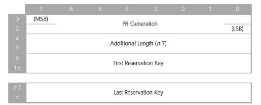
PR Generation A 32-bit counter that is maintained by the drive and incremented every time a PERSISTENT RESERVE OUT command requests a Register, Register and Ignore Existing Key, Clear, Preempt, or Preempt and Abort service action.
