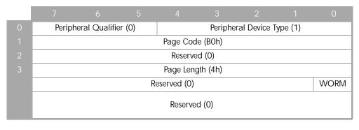
WORM 1 The Device Server supports Write Once Read Many (WORM) operation.
