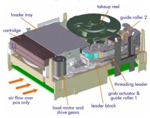
The picture above and the following description refer specifically to a Generation 1 full-height tape drive mechanism, but the principle is the same for half-height and Generation 2 mechanisms.
