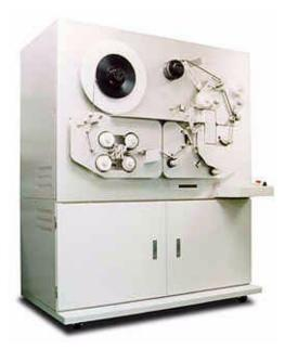
Servo tracks are written during manufacture by an Otari Servo writer, shown on the left. The machine has a very accurate tape path and writes a precise set of five servo tracks down a large spool of tape. The tape is then cut into sections and loaded into Ultrium data cartridges.
