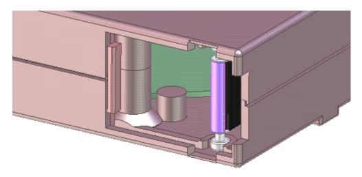
Within the drive, a leader block engages directly onto the leader pin at the end of the tape. It has a spring retainer to maintain the grab in case of power failure or loss of tension.
