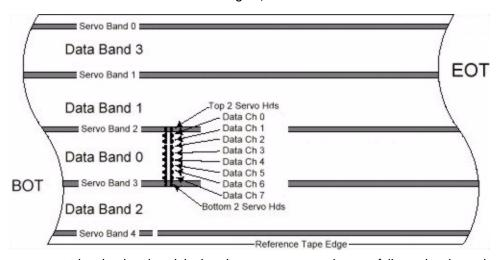
Within the data band the head serpentines, completing a full travel to the end of the tape before changing the head position and writing a track in the reverse direction back down the tape.
