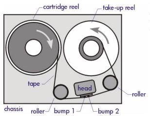
The rotation shown is when reading or writing even-numbered tracks. For odd-numbered tracks, both reels rotate in the opposite direction.
