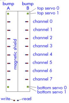
The illustration below shows the actual head assembly. The leading edges are designed to wipe any debris from the tape before it gets to the heads. The tape bearing surfaces are ceramic to resist wear so that the head has a life of >30,000 hrs.
