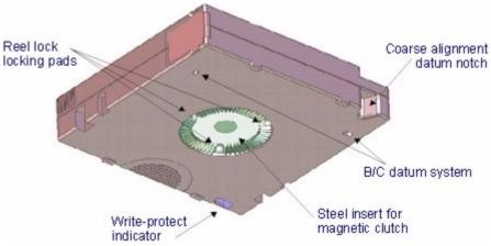
The reel lock locking pads ensure that the reel does not move when the cartridge is not in a drive.
