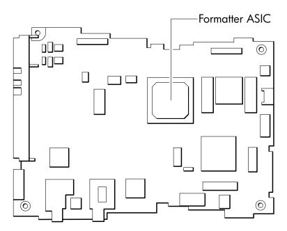
A thermocouple placed on the ASIC should not exceed  $25^{\circ}\text{C}$  over the ambient air temperature while the drive is stream writing for at least one full hour. Thus for an ambient temperature of  $25^{\circ}\text{C}$ , the U6 case lid should remain under  $50^{\circ}\text{C}$ .
