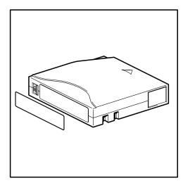
The label and write-protect switch are on the rear face of the cartridge, as illustrated.
