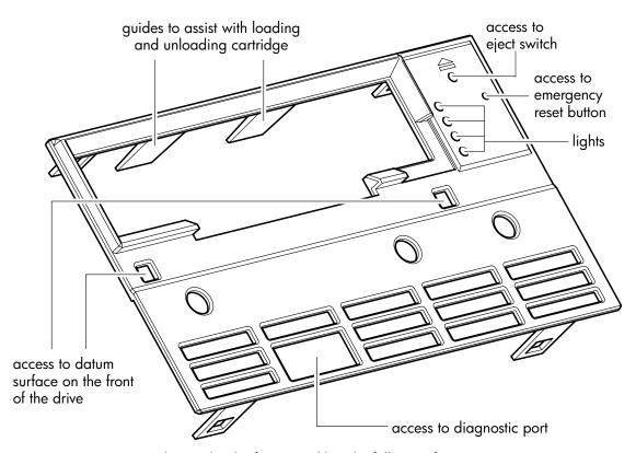
The autoloader front panel has the following features:
