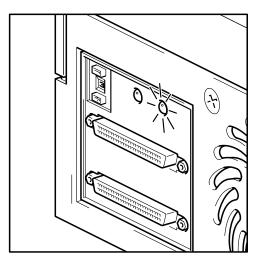
Fan/PWR Fault (fault with the fan or power supply)
