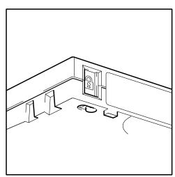
To write-protect a cartridge, slide the red tab by the label area on the rear face of the cartridge to close the hole.
