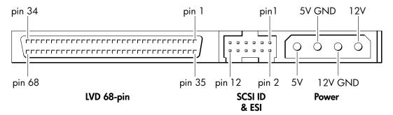
The auxiliary connector is used for setting the SCSI address and potentially as an Enhanced Serial Interface (ESI). The pins are as follows:
