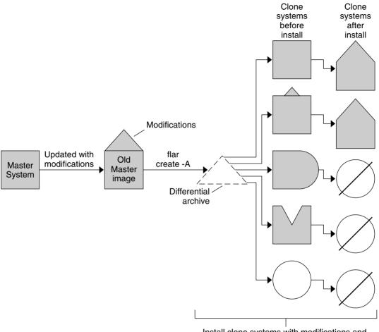
Install clone systems with modifications and validate master and clone system images.
