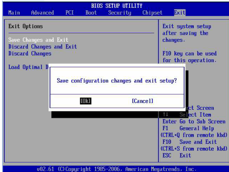
FIGURE E-34 BIOS Setup Utility: Exit - Save Configuration Changes and Exit Confirmation
