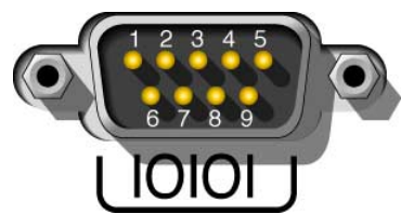
FIGURE A-4 Serial Port (TTYA) Pin Numbering
