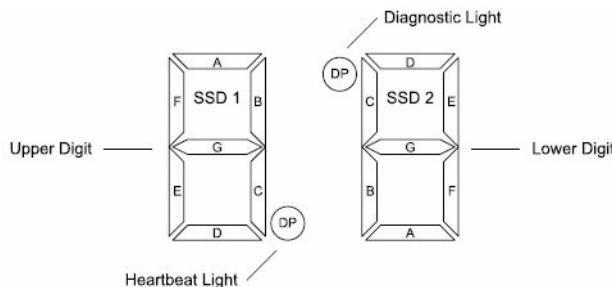
The values on each display (Controller A and Controller B) are shown as if the digits had the same orientation. For example, if the tray ID is set to 43, the top controller display might appear as shown in [FIGURE 5](#), while the bottom controller display would then appear as shown in [FIGURE 6](#).
