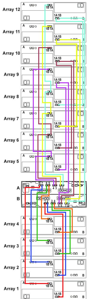
**FIGURE 3** Cabling for One Controller and Sixteen Expansion Trays
