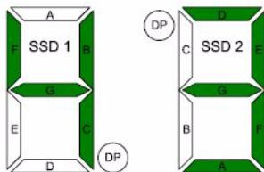
Alphanumeric characters are represented on the display as shown in [FIGURE 7](#). During normal operation, the tray ID display on each controller is used to display the enclosure tray ID. The display is also used for diagnostic codes. The Diagnostic Light indicates current usage. The Diagnostic Light is off when the display is used to show the current tray ID.
