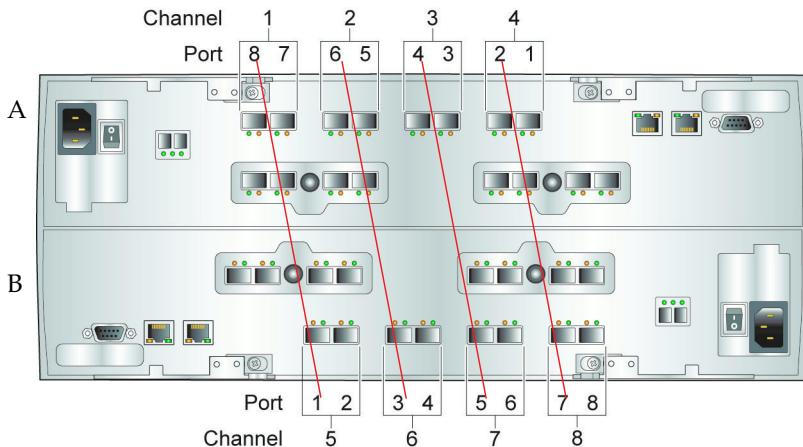
**TABLE 9** Non-sequential Port Connections for Expansion Trays 1 through 7
