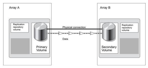
FIGURE 4-1 Relationship Between Arrays and Their Corresponding Replication Sets
