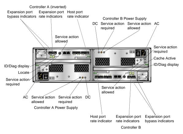
FIGURE 5-2 Controller Tray LEDs and Indicators (Back View)
