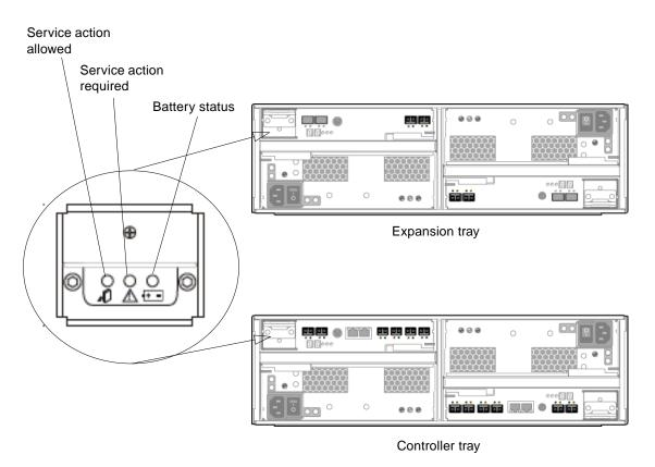
FIGURE 5-4 Battery Compartment LEDs
