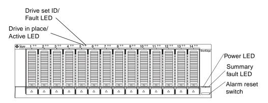
FIGURE 1-5 LEDs on the Front of the Sun StorageTek 6130 Array Controller Tray
