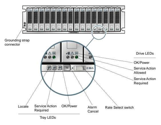
FIGURE 5-1 shows the LEDs and components on the front of the controller tray.
