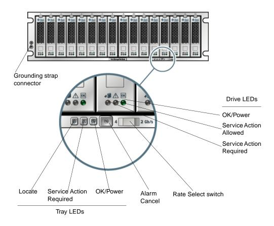
FIGURE 1-2 Sun StorageTek 6140 Array Controller Tray (Front View)
