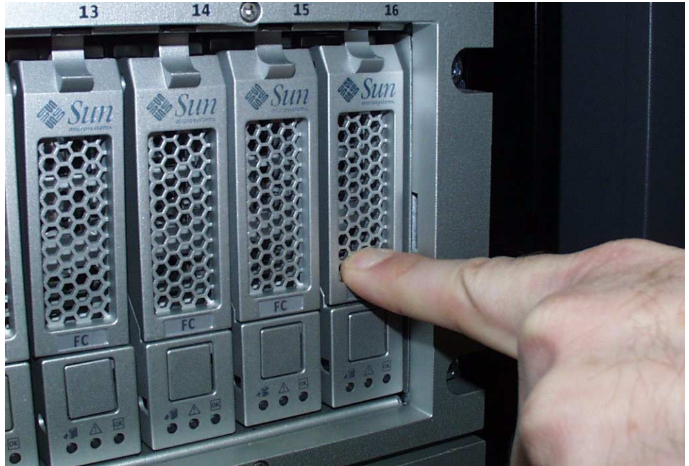
FIGURE A-2 Successfully Inserted Disk Drive
