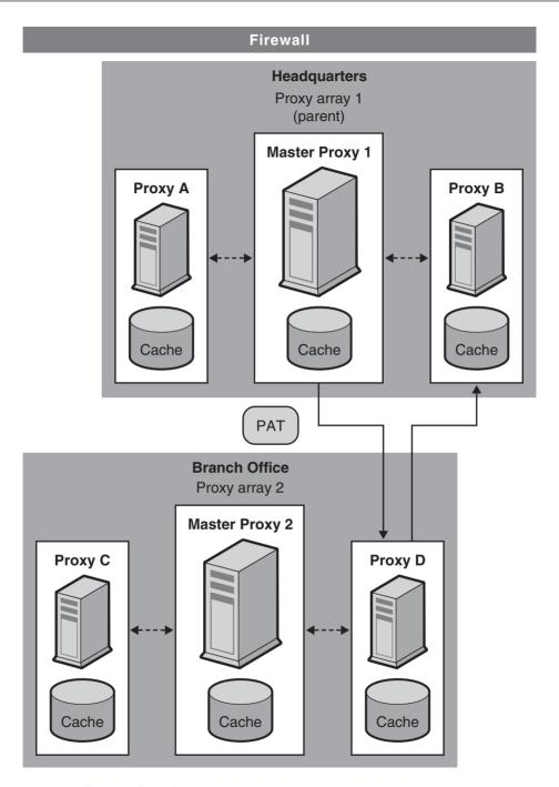
FIGURE 12-5 Proxy-to-Proxy Routing
