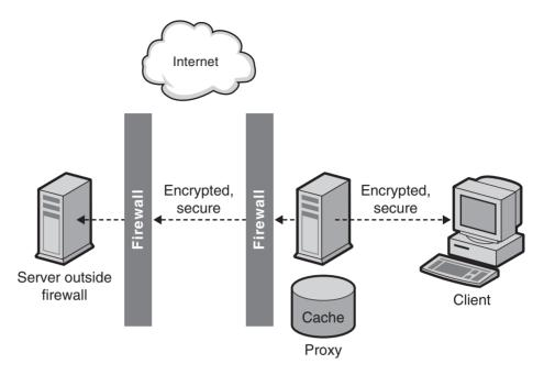
FIGURE 14-4 Secure Client Connection to Proxy and Secure Proxy Connection to Content Server
