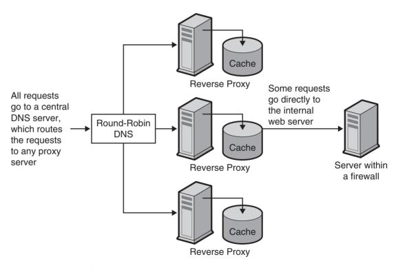
FIGURE 14–5 Proxy Used for Load Balancing
