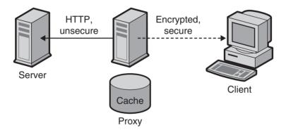
FIGURE 14–2 Secure client connection to proxy
