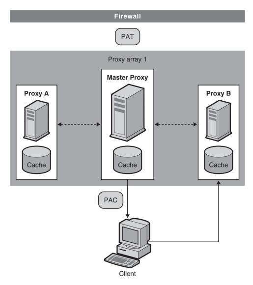
FIGURE 12-4 Client to Proxy Routing
