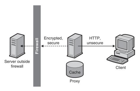
FIGURE 14-3 Secure Proxy Connection to Content Server
