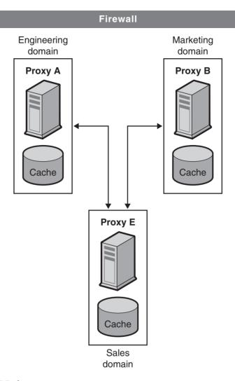
FIGURE 12-3 ICP Exchange
