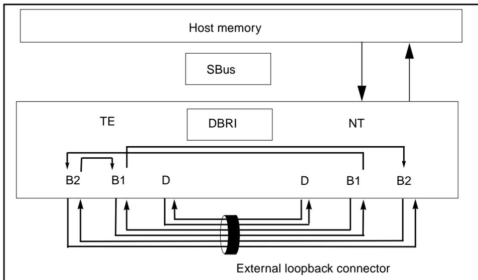
**FIGURE 24-4** isdntest Data Path Subtest
