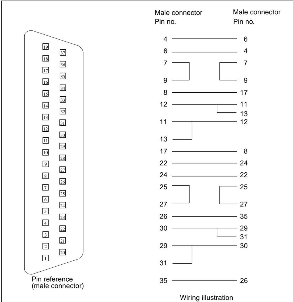
**FIGURE A-9** 37-Pin RS-449 Loopback Cable
