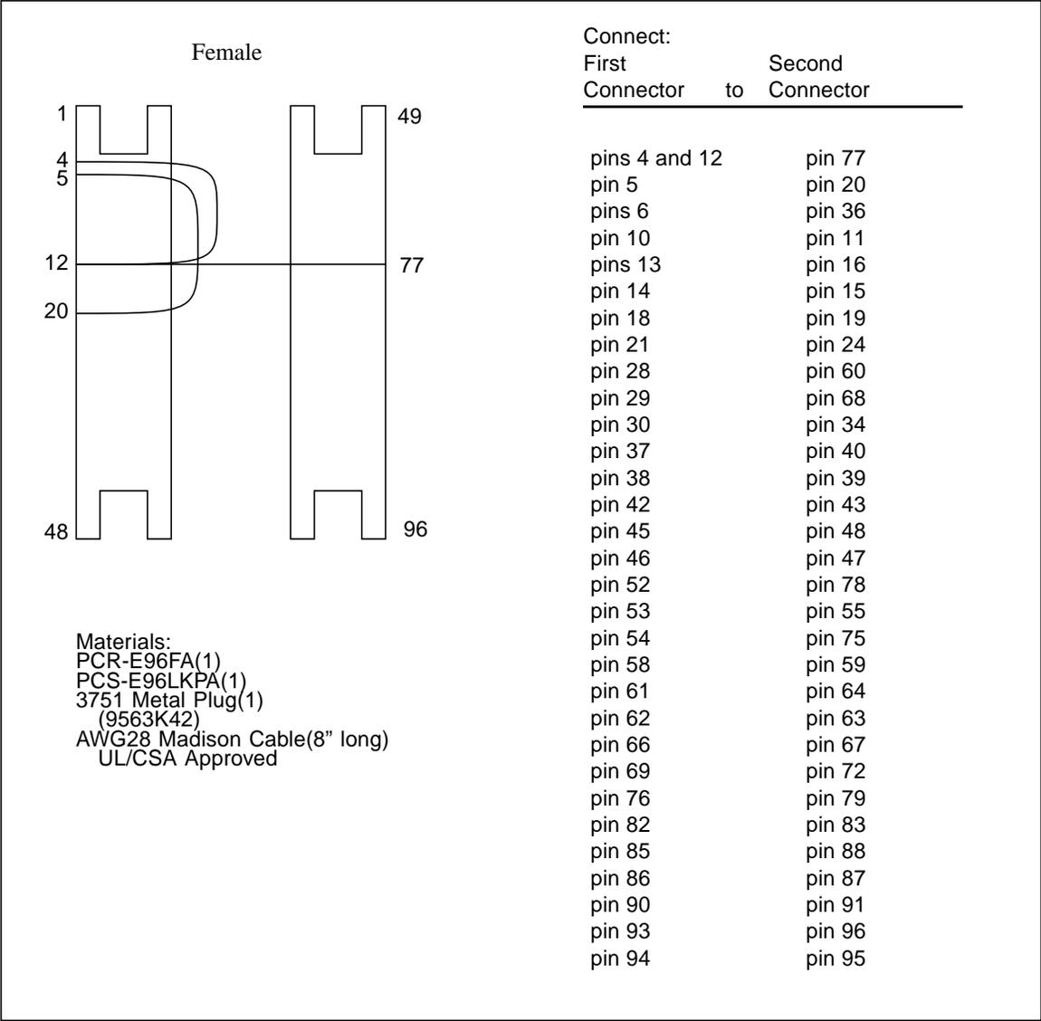
**FIGURE A-7** 96-Pin Female Loopback Connector
