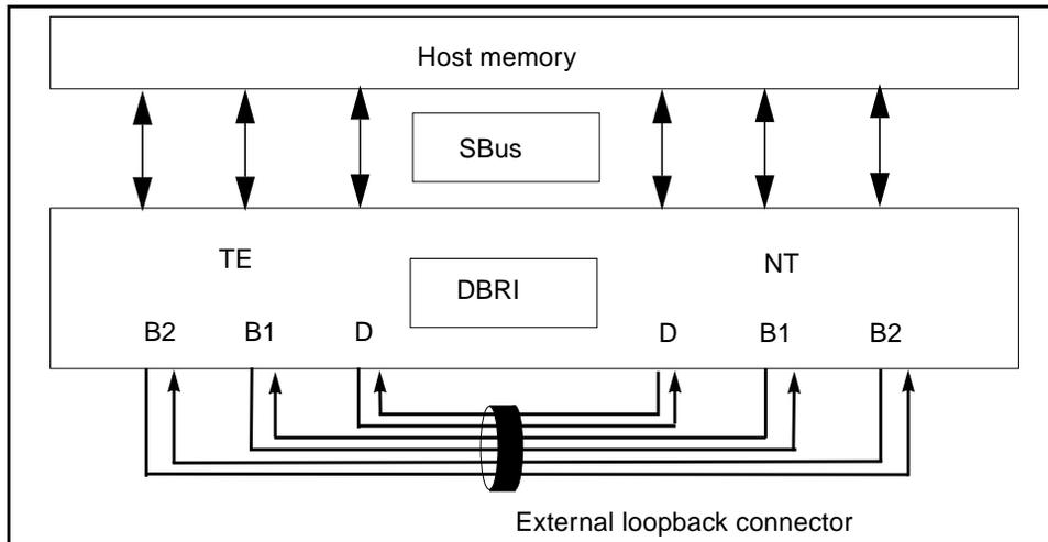
**FIGURE 24-3** isdntest Read/Write Subtest
