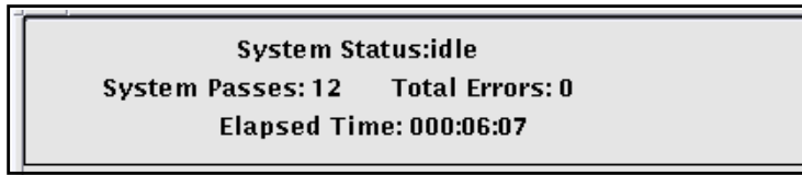
FIGURE 5-2 OPEN LOOK Status panel
