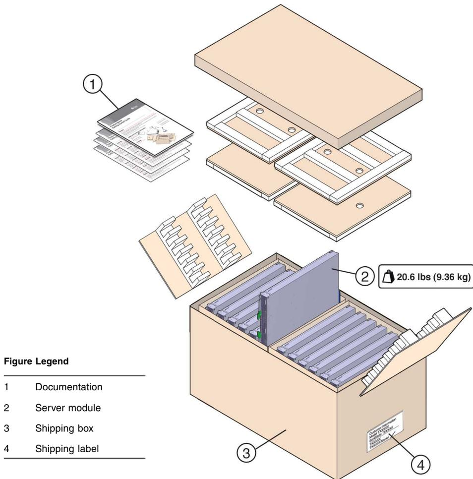
**FIGURE 1-2** Shipping Box Contents (Single Blade)
