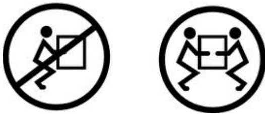
FIGURE: Lift Warning
