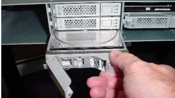
FIGURE 2 Inserting the Drive.
