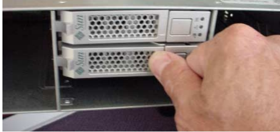
FIGURE 4 Fully Inserting the Drive.
