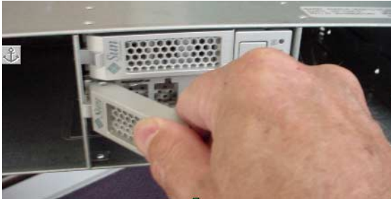
FIGURE 3 Pushing the Disk Drive Latch.
