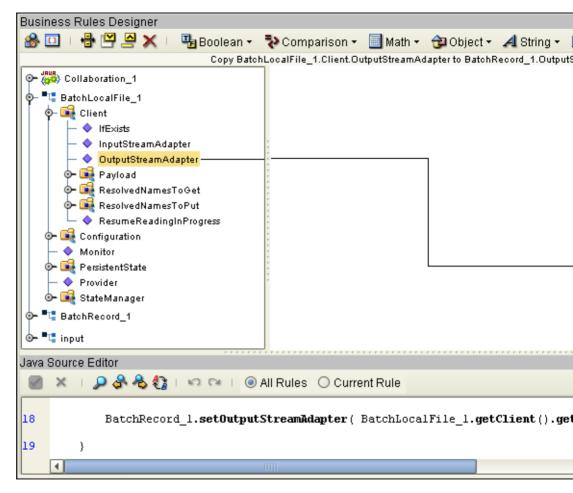
■ Transfer data from a local file system (BatchLocalFile) to a remote FTP (BatchFTP) setup. This scenario uses the **InputStreamAdapter** OTD node (see "Data Streaming Scenarios" on page 10).
