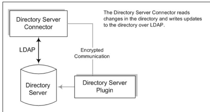
FIGURE 4-4 How Directory Server Connectors Detect Changes
