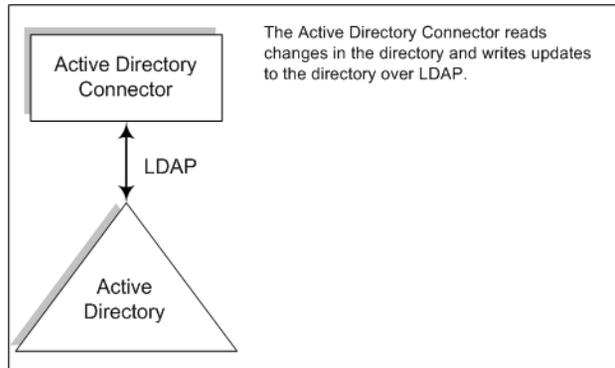
FIGURE 4-5 How Active Directory Connectors Detect Changes
